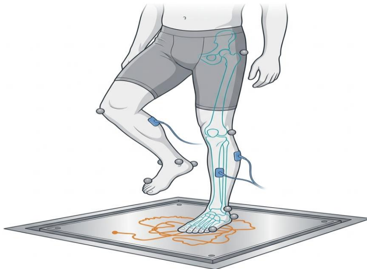
Figure 2: Experimental Setup and Biomechanical Modeling for Unilateral Stance Assessment on a Force Platform
